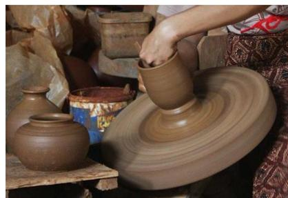
Gambar 3. Perbot miring tampak samping
